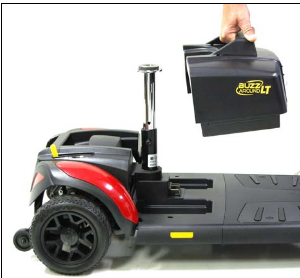
Figure 21. Battery Pack Installation
