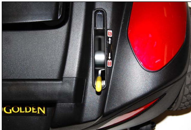
Figure 11: Freewheel Lever (Drive Position)
