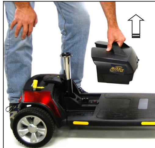
Figure 15. Removing the Battery Pack
