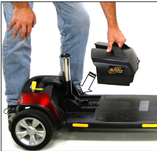
Figure 21. Battery Pack Installation
