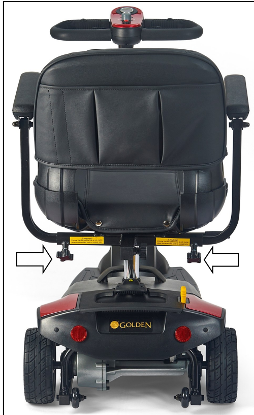
Figure 6. Armrest Width Adjustment
