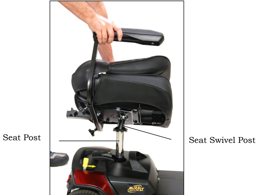
Figure 23. Installing the Seat
