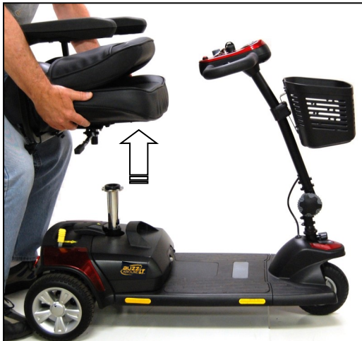
Figure 14. Removing the Seat
