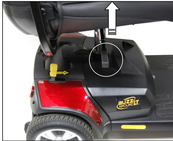
Figure 8: Seat Rotation Adjustment
