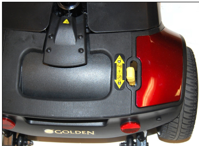
Figure 11: Freewheel Lever (Drive Position)
