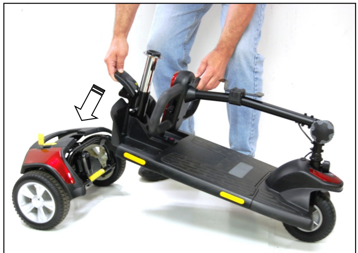
Figure 20. Connecting Frame and Drivetrain
