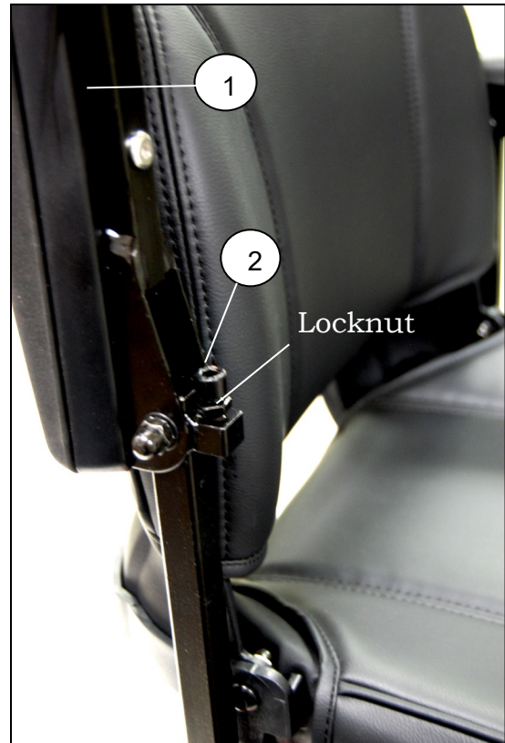
Figure 7. Armrest Angle Adjustment
