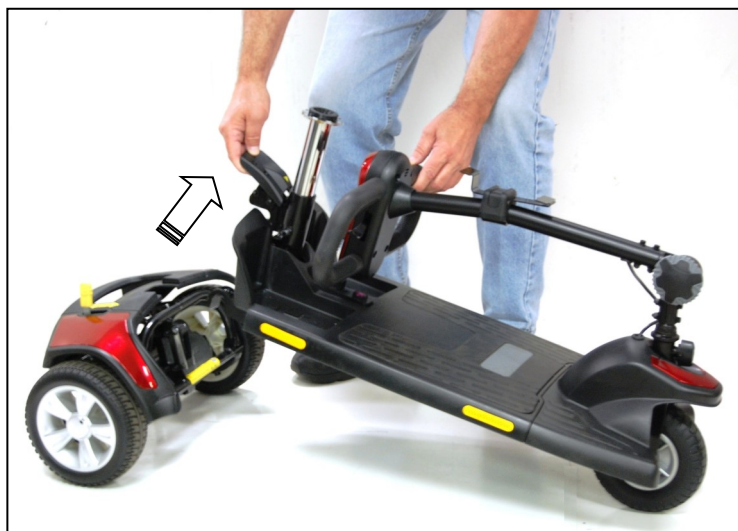
Figure 17. Separating the Drivetrain and Frame
