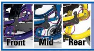
The unique **Tilt Assist** feature makes tilting easier by reducing the effort required to tilt an occupied Solara 3G or Spree 3G wheelchair by 30%. With three settings, front, middle and rear, the simple Tilt Assist adjustments help to correct for uneven weight distribution caused by seating systems and other components.
