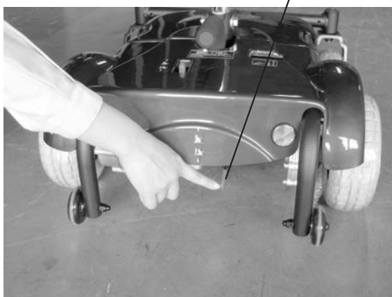
Fig J. Move release bar downward to freewheel mode. (Left motor)
