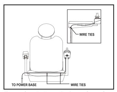
Figure 11. Controller Harness Routing on a Contour Seat
