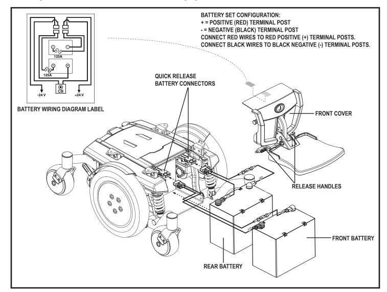
Figure 24. Battery Installation
