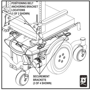
Figure 12. Transit System Securement Brackets (Synergy Seat Shown
