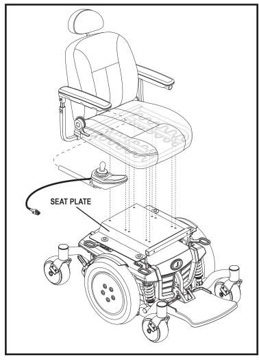
Figure 10. Seat Installation-UK Occupied Transit Securement System
