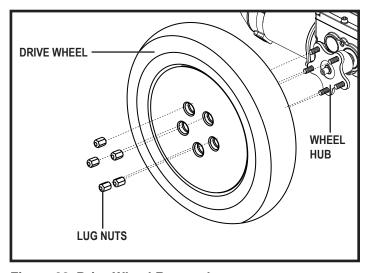
Figure 23. Drive Wheel Removal
