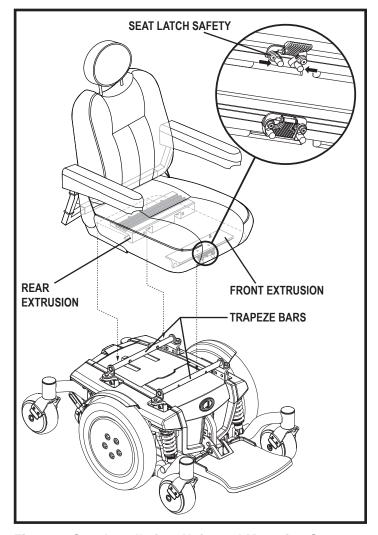
Figure 8. Seat Installation-Universal Mounting System
