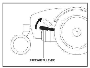
Figure 4. Drive Mode (Drive Engaged)
