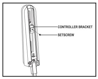
Figure 19. Underside of Armrest
