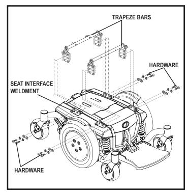
Figure 15. Seat Height/Angle Adjustment-UMS
