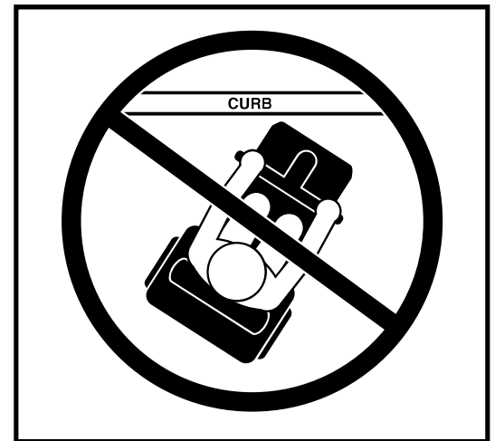
Figure 7. Incorrect Curb Approach
