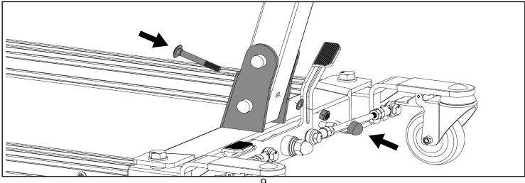
Step 4: Insert the round plastic cover and the large plastic washer to the boom as follows.
