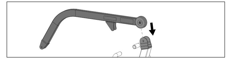
Step 6:Secure the boom to the mast by reinstalling the bolt, washer and nut. Once the screw is tightened, reinsert the plastic cap.
