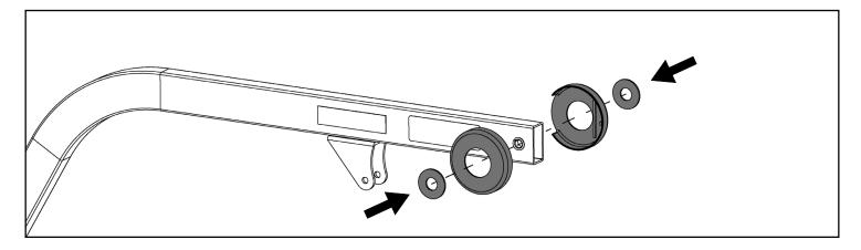
Step 5: Install the boom to the mast bracket, and make sure the plastic cover and plastic washers are still attached to the boom.
