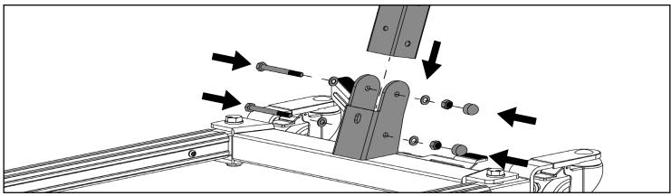
Step 3: Insert the carriage bolt to the front hole of the bracket, and secure the mast using bolts and nuts as follows, reinsert the plastic cap after the screw is tightened.
