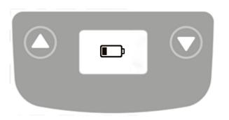
If the battery needs to be charged, the LCD Display Panel will show a blinking low battery sign shown on the left either when the emergency stop button is released or when a button on the LCD Display Panel is pressed.
