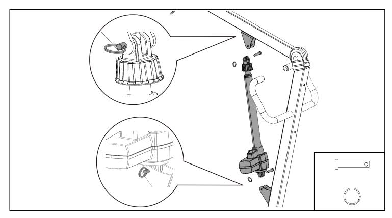
Step 8: Secure the spreader bar to the boom using a pin and retaining ring as follows.
