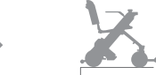
Do the same for the rear wheels to get the device over the step.
